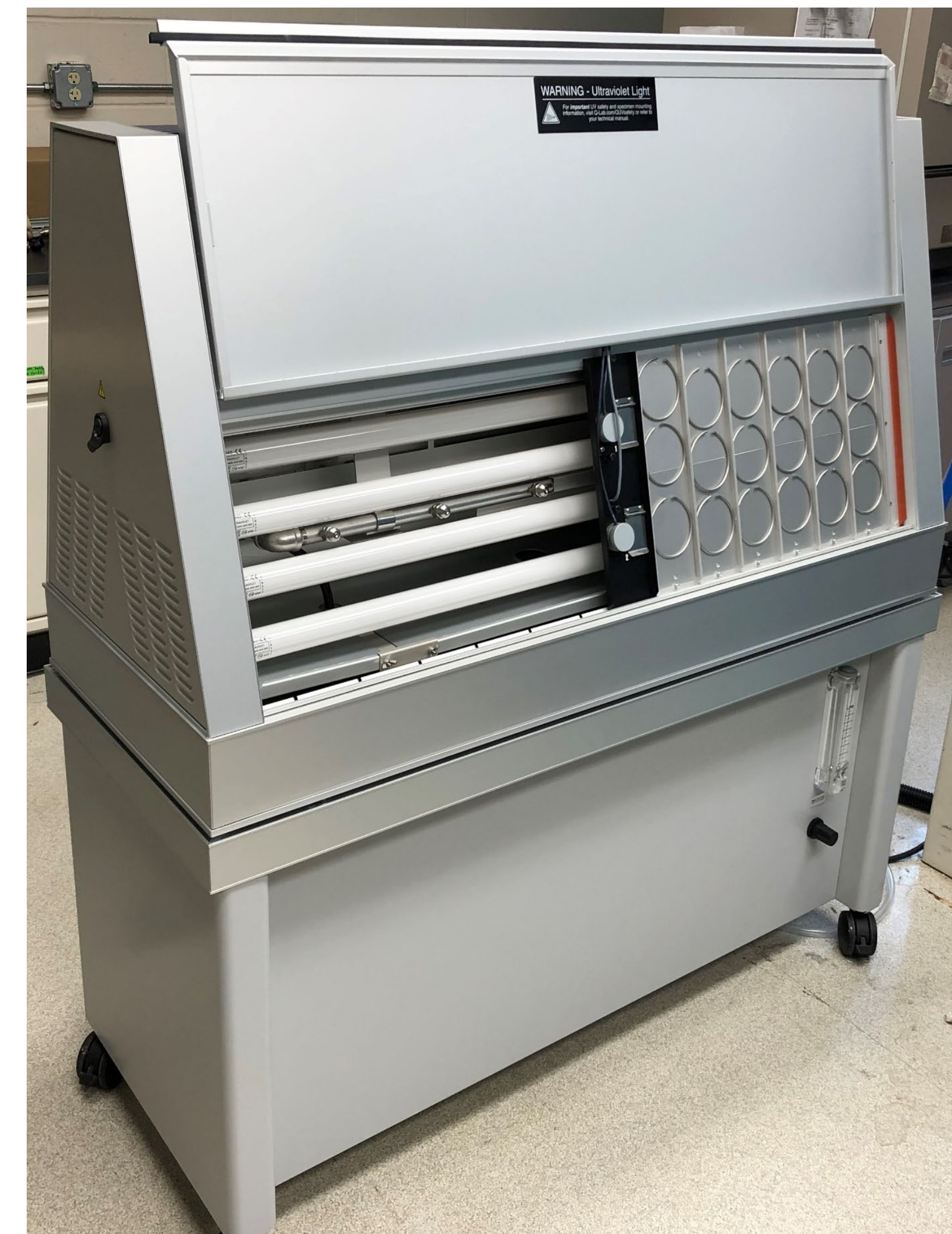
Figure 2. Q-Lab QUV Spray Accelerated Weathering Tester
