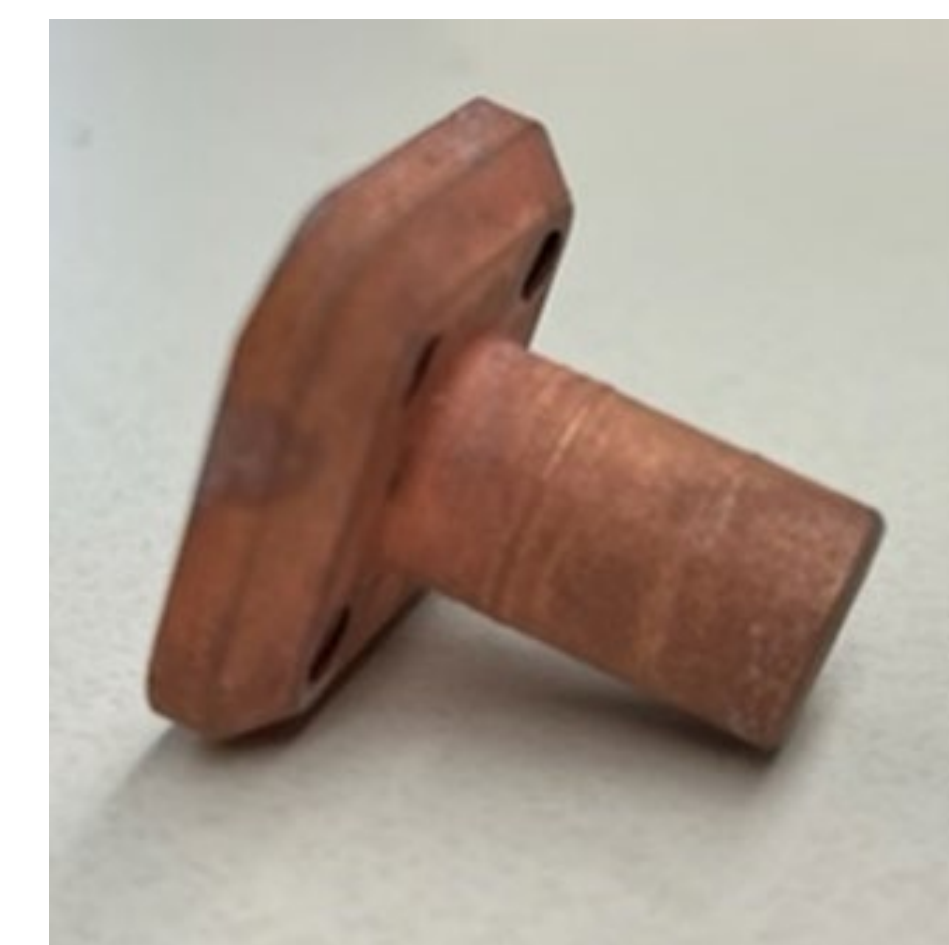
Copper Plated Polymer Part
