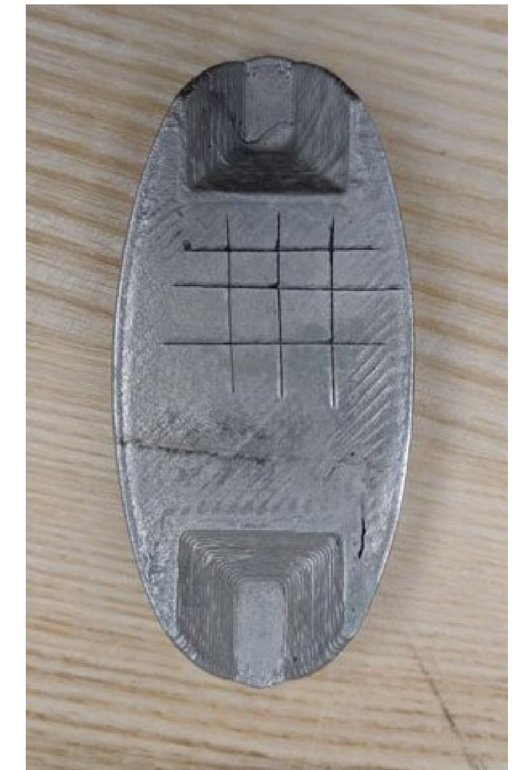
Nickel-Coated Part Subjected to Scribe-Grid Test
