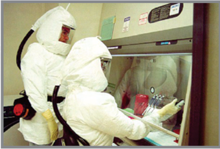
Virus isolation by tissue culture performed in biosafety cabinet in BSL3 laboratory.
